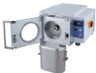
The universal 2 in 1 mill for dry products
